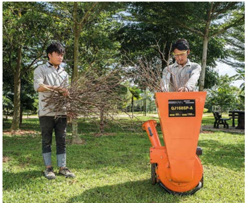
Shredder machine to crush trimmed branches and natural waste to be reused as organic fertiliser for the landscape
